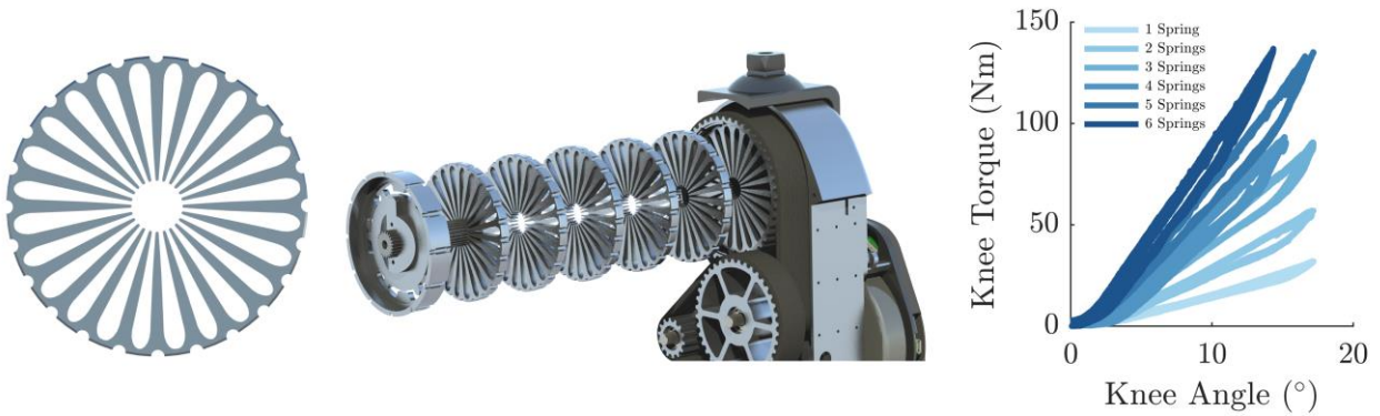
Fig. 3. Front view of an individual spring disk (left), exploded view of the spring disks stacked inside the knee output pulley (middle), and torque-angle relationship of the knee at various levels of series elasticity (right).
